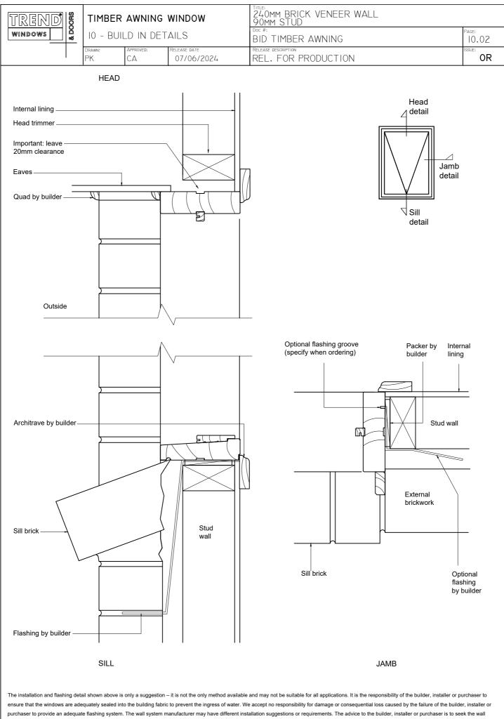
system manufacturer's requirements for installation and flashing and to seek clarification from the wall system manufacturer if different.
