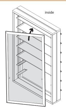
4. Bring flyscreen in and pull up the top of the screen so that the head clips grip the top bead.
