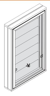
third floor level, tie a light nylon cord to the lift tabs to secure the screen so that it is not damaged or causes damage if it is dropped
