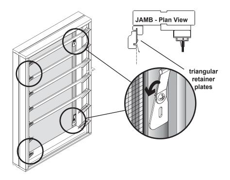
5. At each of the triangular retainer plates, use the plastic handle and rotate the clips into recess.
